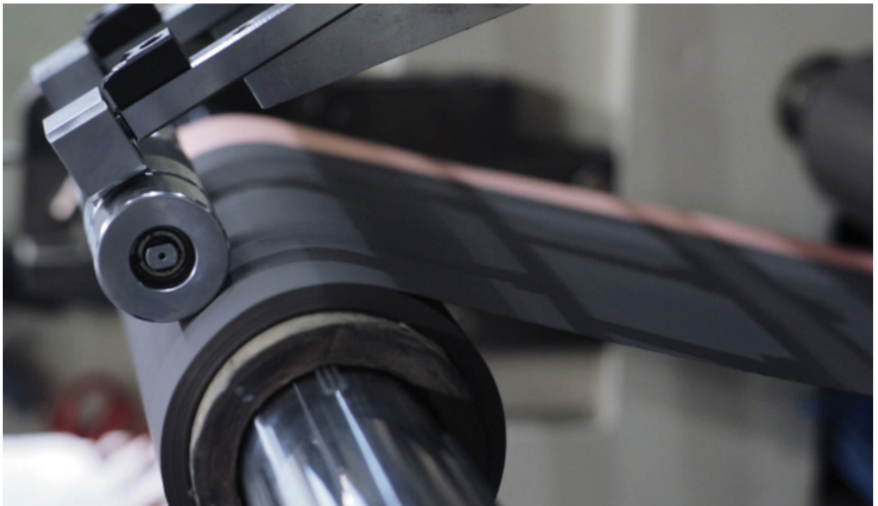
FIGURE 1. The battery coating process. (Courtesy of Teledyne Vision Solutions)
